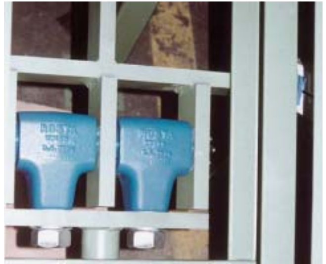
Drive head fixation on chip feeder
