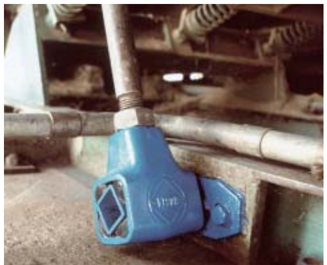
Rocker fixation on feeder frame
