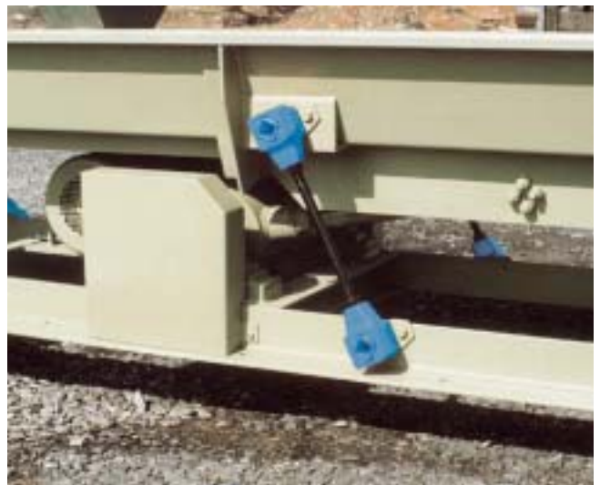
Single rocker on chip feeder
